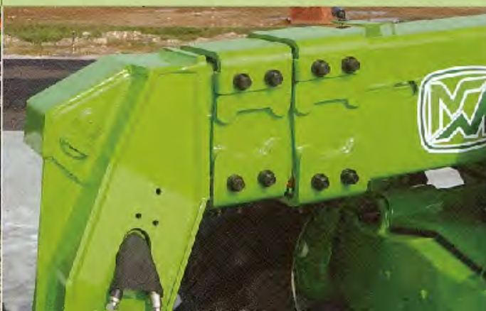
Boom sections slide on adjustable low-friction pads
