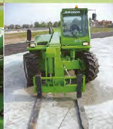
The 'disappearing' boom ensures an excellent 360° visibility.
