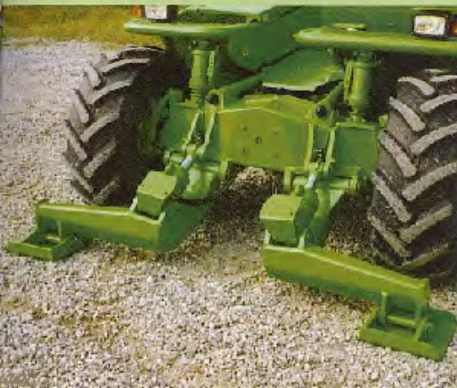
The front stabilisers assure the necessary stability for working on any terrain.
